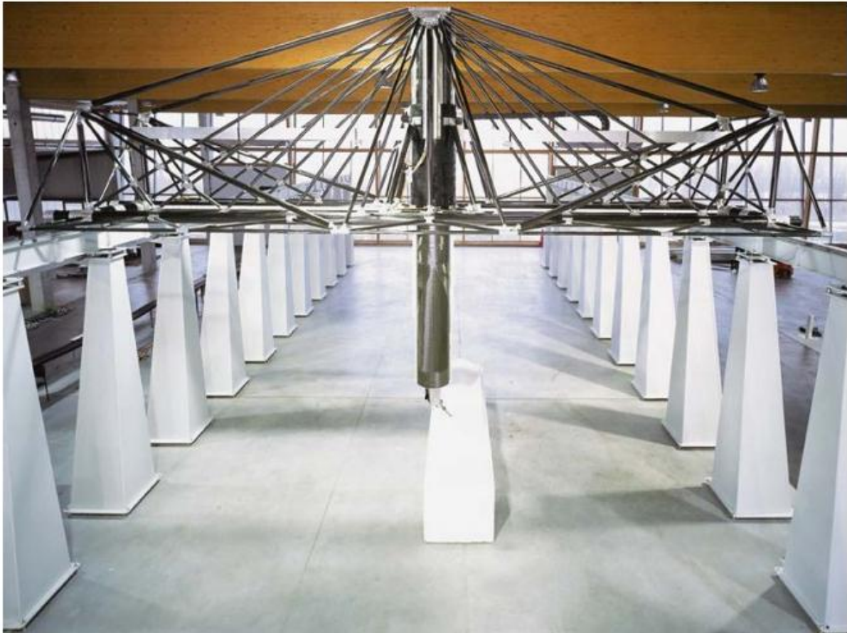
HSM-Modal at rest. The carbon fiber components allow the machine to sit nimbly on a series of small posts. Photo: EEW Protec
